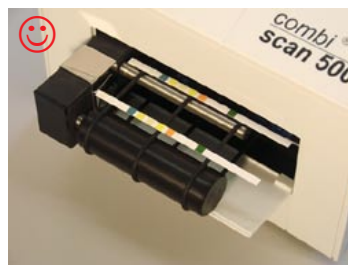
The strips move automatically to the optical unit.
